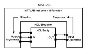
The following figure shows how a MATLAB component function is wrapped around by and communicates with the HDL simulator during a component simulation session.
